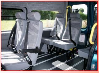
Our standard specification includes fully bonded glazing to manufacturer's specification, luxurious, but hardwearing trim, M1 and M2 tested passenger seats (all fitted with integral lap and diagonal belts) which conform to the latest EEC Directives. An extensive list of options is available to enable the discerning customer to bespoke their minibus to meet their specific requirements.
