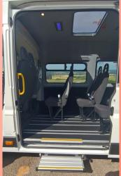
Entry is through a full height side door which gives easy passenger access. A variety of tail-lifts is available for wheelchair and
